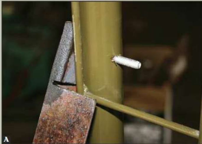
A bolt attaches the bracket to the door frame (A). Once attached, rope or chain provides support to the bracket (B).
