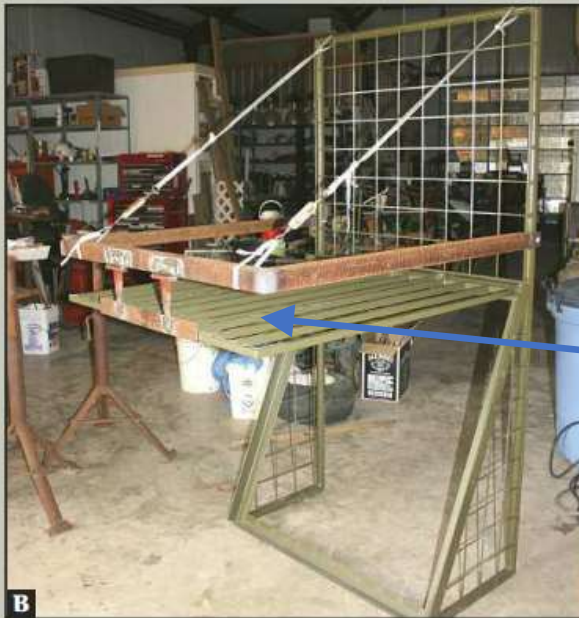
A bolt attaches the bracket to the door frame (A). Once attached, rope or chain provides support to the bracket (B).
